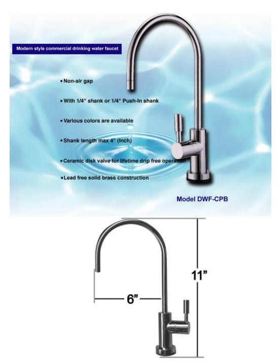
Mounts on standard sink hole (1 3/8") or  $\frac{1}{2}$ " hole. 3/8" push-fit faucet connector included. Polished chrome brass faucet supplied for the Starwood Hotels element units.
